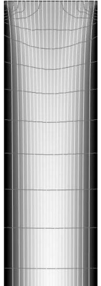
Simulated channel entrance flow at \operatorname{Re} = 100 . The fluid enters on top and exits at the bottom. Note how the streamlines (light) converge towards the center while the pressure contours (dark) flatten out as the Poiseuille profile is established downstream.
