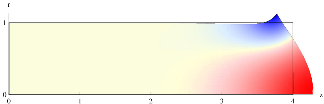
Figure 9.1 page 142. Demonstration of Saint-Venant's principle. A circular cylinder with radius a = 1 and length L = 4 is placed with its z -axis as shown. You should rotate the figure around the z -axis to see the three-dimensional image. The originally relaxed cylinder is loaded at the right end with a radially varying pressure distribution p_z = -\sigma_{zz} = 2r^2 - 1 , for which both the total force and total moment of force on the cylinder vanish. Young's modulus is taken to be 1000, and Poisson's ratio 1/3 . The colors indicate the pressure p_z along z in the cylinder, with red being positive (compression) and blue negative (extension). The pressure distribution is seen to extend less than one diameter from the right end, in accordance with Saint-Venant's principle. The surface deformation is strongly exaggerated.
