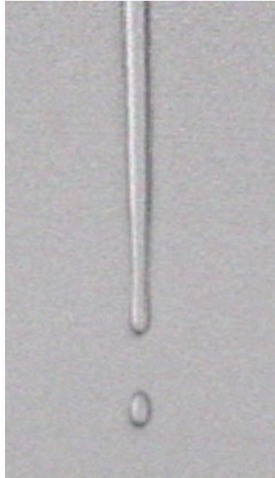
FIGURE 3. The tip of the surface depression is unstable when the rotation rate of the container is high. An air-bubble with radius of about 0.5 mm has just detached from the tip and is dragged down the drain by the surrounding flow. The photograph was made with a preliminary setup.
