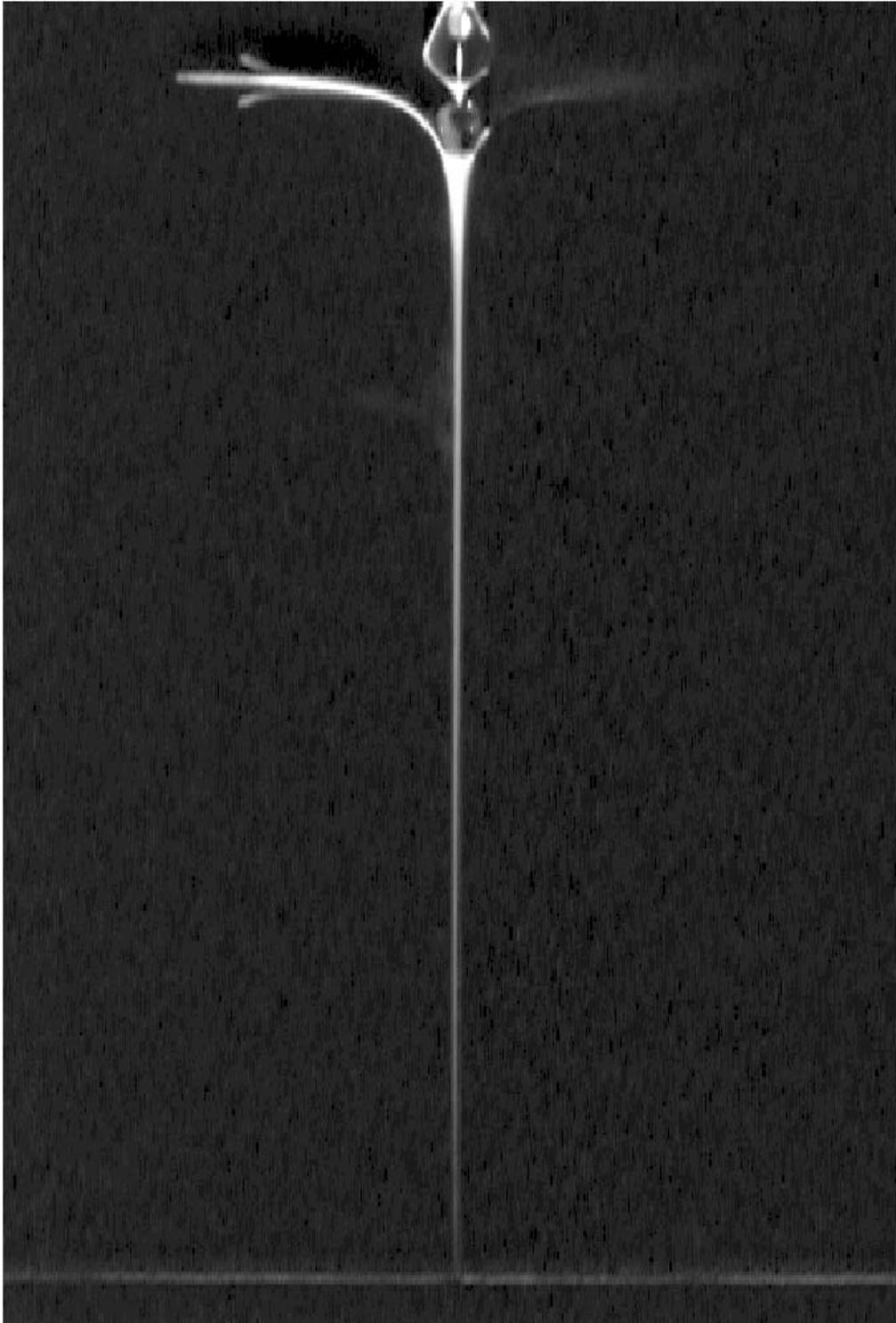
FIGURE 4. Visualization of the downward flow in the vortex core above the drain-hole at 12 rpm. The dye was added at the surface and is flowing in a free surface boundary layer to the core region where it flows rapidly down-ward to the drain-hole. The top part of the image shows reflections in the free surface which are artifacts of the method of observation.
